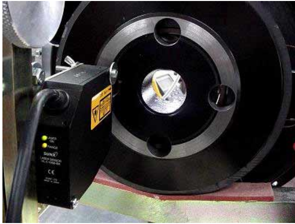
Figure 21: Measurement of the coil motion using drilled holes on the magnetic back plate in a loudspeaker which has a wider air gap.
