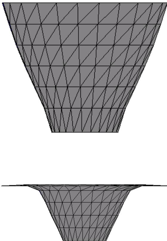
Figure C1: Upper: Mode 73 (1143 Hz) of a truncated cone restrained by the neck. Observe the main longitudinal motion due to in plane deformations. Lower: Mode 116 (1621 Hz). Observe the main radial motion due to cone rim bending.
