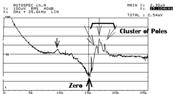
Figure 24: In vacuo motional impedance measurements of a dome compression driver of large voice coil.
