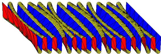
Figure A6: Mode 7 of the pleated tweeter of Figure A5.
