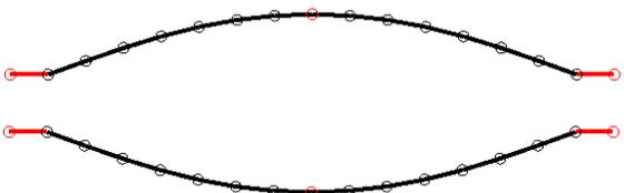
Figure 5: Dynamic response. First mode of the beam of Figure 1 when beam it is restrained by its ends but not by the beam's suspension.
