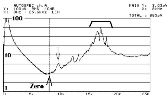
Figure 25: In vacuo motional impedance measurements of a dome compression driver of large voice coil after 5 hours in the vacuum chamber.
