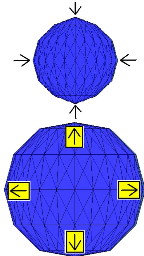
Figure 12: Sphere orthotropically suspended by its equator, performing the breath mode. Generalized mass calculated is 14.37 grams.
