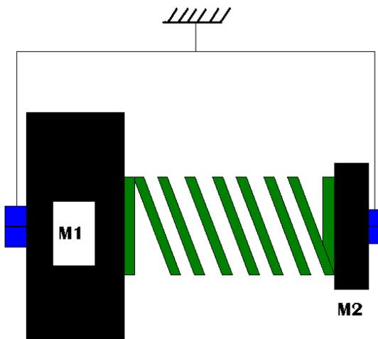
Figure 22: Experimental two degrees of freedom system for driving point mobility measurements.
