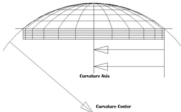
Figure 16: Spherical segment and cylinder which curvatures are at the same side.
