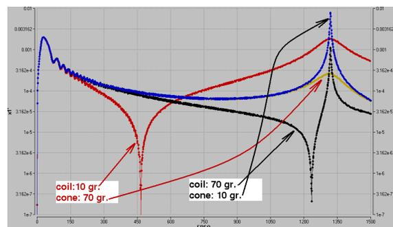
Figure 21: Velocity spectra of a light (10 grams) and heavy (70 grams) voice coil attached to its associated cone. The moving assembly has a fixed total mass of 80 grams. Velocities of the associated cones are depicted as well.
