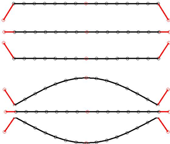
Figure A3: First and second target mode of a round suspended beam loaded by its own weight.
