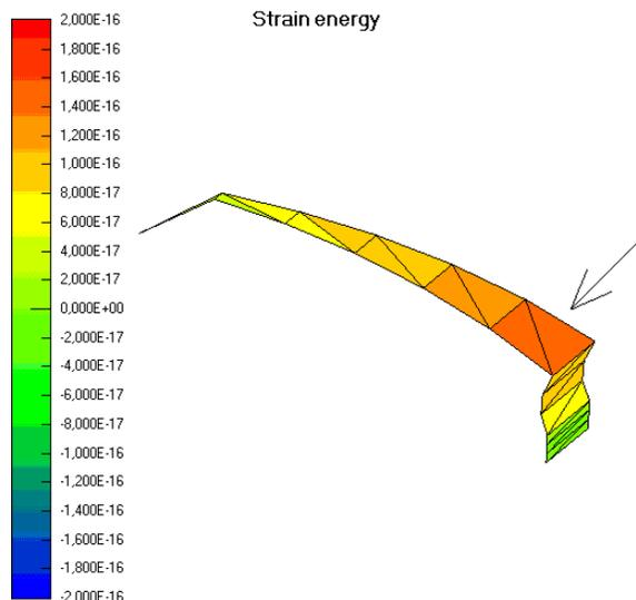
Figure 8: Strain Energy diagram for the deformed moving assembly of Figure 7. Arrow shows the element with highest strain energy
