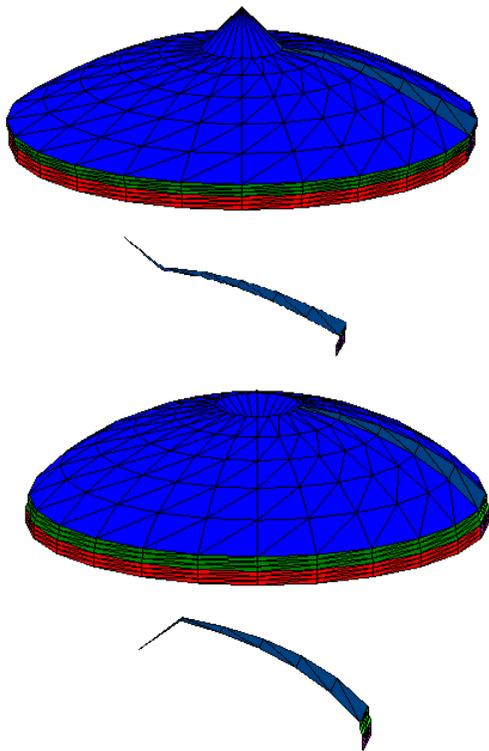
Figure 18: Spherical segment and cylinder performing an axial mode. Dome is bending but the coil's former it is bending and stretching as well. See the explanations of pole bending on text.
