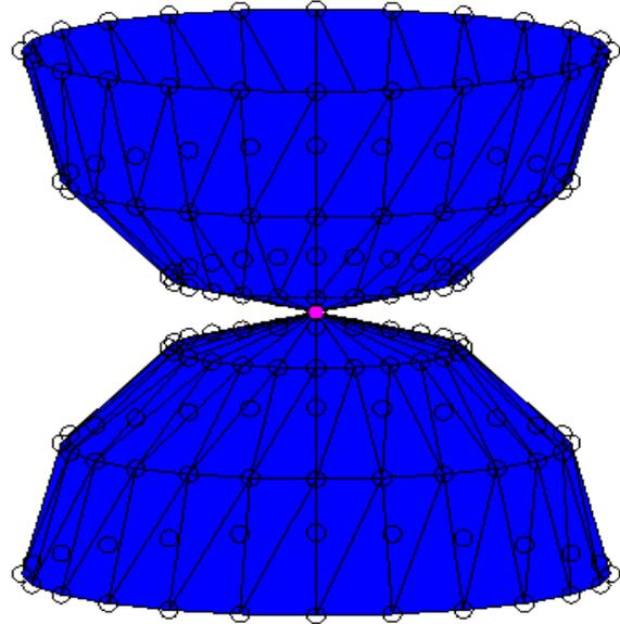
Figure 10: Finite element mesh of the theoretical device of Figure 9. Body is suspended isotropically by the interface node. Model is at rest.
