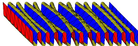
Figure A5: Main motion (mode 2) of the pleated tweeter of Figure A5.
