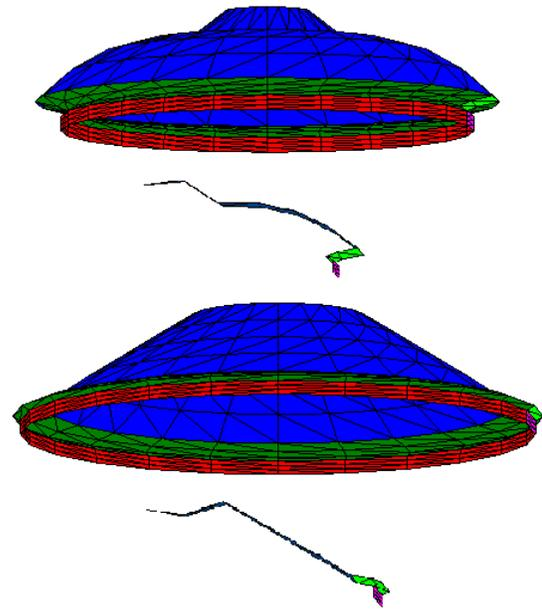
Figure 17: Spherical segment and cylinder performing a compound breathing mode. Observe the coil's ring motion.
