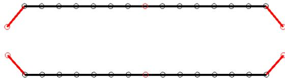
Figure 4: Dynamic response. First mode-shape of the beam –suspension set of Figure 1.
