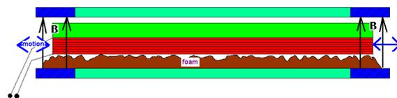
Figure 14: Coil submitted to an axial magnetic field while intensity is circulating. Forces are radial and the body is vibrating “breathing”. The body below the voice coil it is soft foam.
