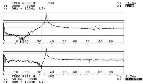
Figure 23: Driving point mobilities of the two degrees of freedom system of Figure 22. Upper: mobility of the light mass. Lower: mobility of the heavy mass.
