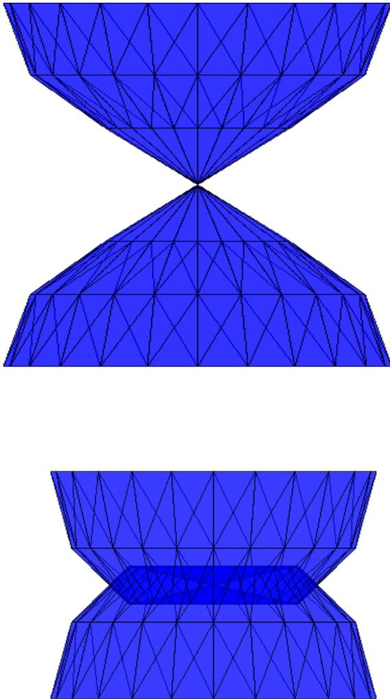
Figure 11: Top: Main mode of the compound body of Figure 12. Middle and Bottom: Axial mode of this body. The generalized mass calculated for this mode is 14.04grams.
