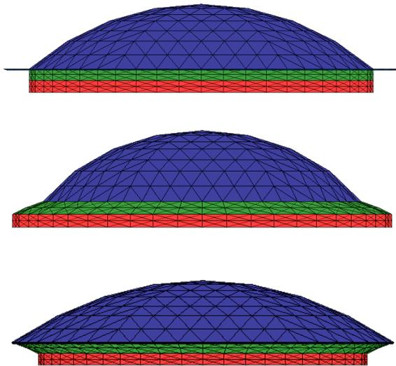
Figure 26: Top: Moving assembly with its suspension. Bottom: Effect of the suspension's radial forces on the moving assembly (suspension is omitted on illustration for clarity).
