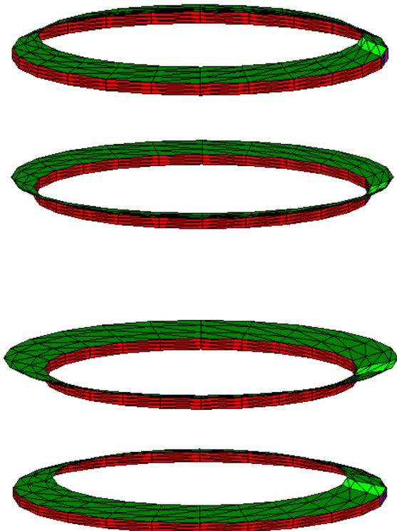
Figure 13: Upper Breath mode of the coil’s former. Lower: Breath mode of the coil.
