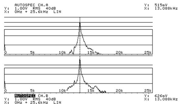
Figure 15: Radial acoustic response on the near field of an aluminum coil with its former. Coil’s diameter is 100 mm, and the coil’s height is 5 mm. Coil’s breath sound was measured by two microphones arranged radial 90 degrees apart.
