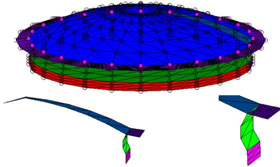
Figure 7: The moving assembly after loaded by its own weight. The body is restrained in translation for all degrees of freedom at the dome-former interface (these nodes are highlighted). Observe details of the deformed former and the dome's pole in the inset.
