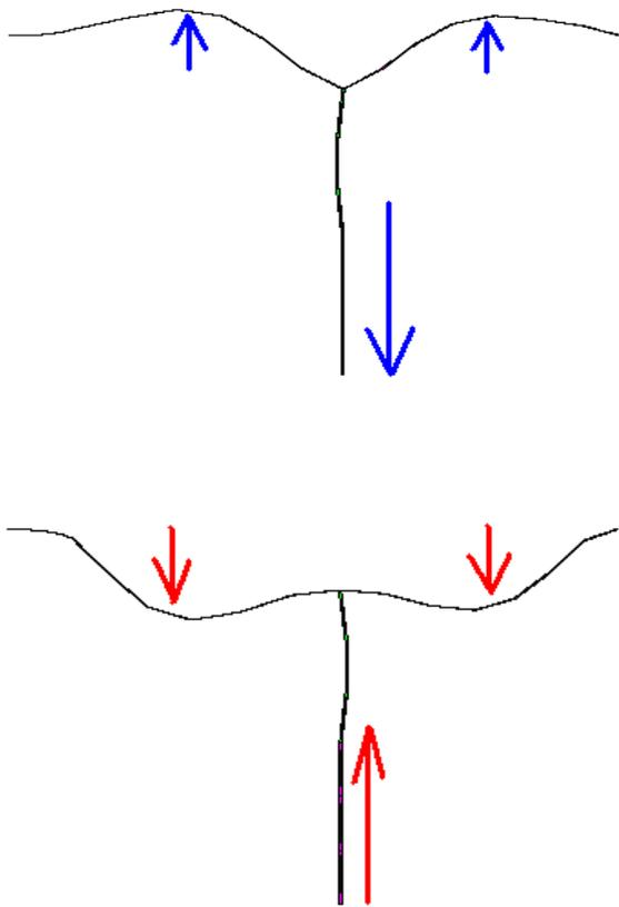
Figure B2: Upper: Main target mode of a V shape transducer with a flat suspension. Lower: Second target mode of the moving assembly. Only right side is depicted for clarity.
