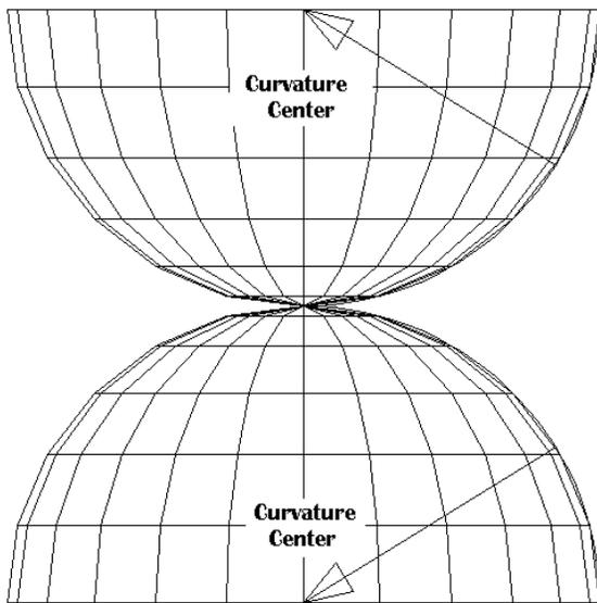
Figure 9: Two hemispheres jointed by its poles. This is an example of a compound body, with curvatures in opposition. The body is suspended isotropically by the common node.
