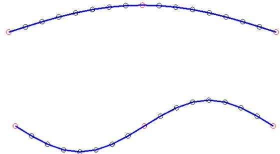
Figure A2: First and second mode of the beam loaded with the masses of Figure A1.
