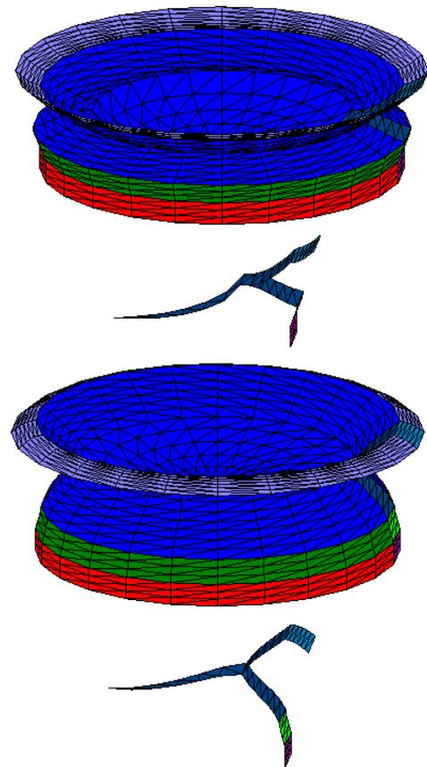
Figure 20: Main axial mode of the moving assembly of Figure 19.
