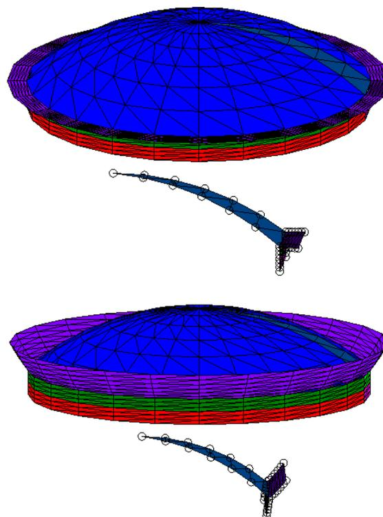
Figure 6: Upper: Coil, Former and Dome of a compression driver with its suspension. Bottom: Shape of the moving assembly after loaded statically by its own weight.
