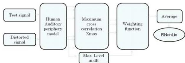
Figure 2 Block diagram for the Rnonlin calculation process.
