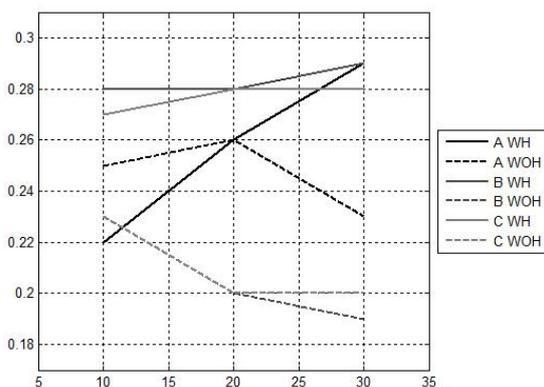
Figure 5 Roughness vs input voltage obtained for the three devices with and without horn.
