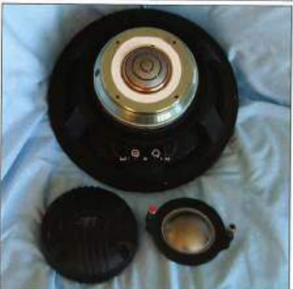
Photo 2: Cooling for 12CX4400Nd is primarily provided by the motor mass and the black finned compression driver cover.
